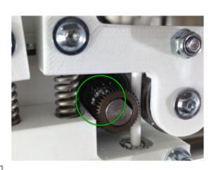
Filament abrasion at the drive gear due to
