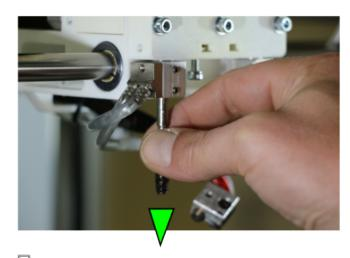
Pull the barrel out of its seat.
