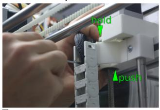
Hold down the pulley and push up the clamp collar.
