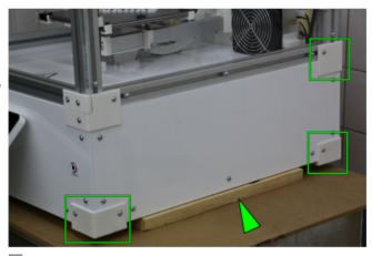
Lift the 3D Printer at one side; the feet and the hind cover angle must be removed.
