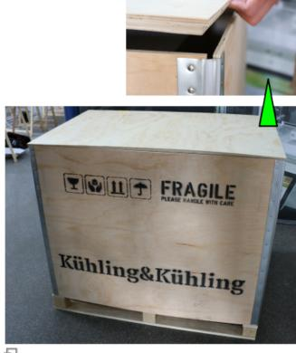
Ensure the lid fits so that tensioning the lashing straps will work.
