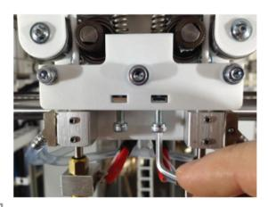
Adjusting the idler lever preload.
