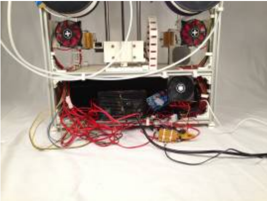
Back view - cable harness waiting for new high power MOSFET driver boards to be finally wired up
