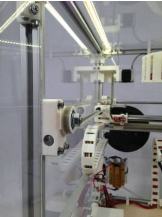
Front left Y end with belt idler
