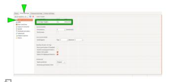
First layer height and support material extruder nozzle diameter must correspond.
