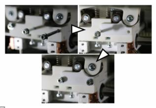
Installing the adapter for flexible filaments.
