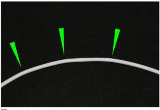
Solution States in the filament may also lead to jamming.
