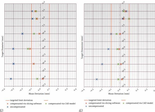
The deviation decreases significantly when the thermal expansion is compensated. Either for diameters of circular structures ...
