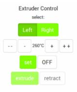
Try finding the suitable temperature by directly extruding via the *Expert Control* screen.
