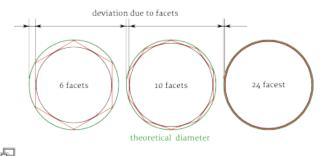
In case of roughly faceted objects try increasing Correlation of low faceted walls and diameter. the resolution of your CAD model to improve dimensional accuracy.
