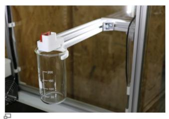
The Wiper Upgrade Kit provides the necessary hardware for successfully printing dual extruder print jobs.
