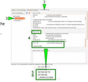
Switching off the build chamber heating elements by modifying the Slic3r custom End Gcode.
