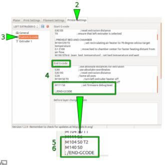
Switching off the build chamber heating elements by modifying the Slic3r custom End G-
