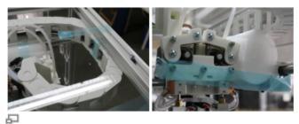
Transport restraint of the main e-chain: blue tape is strapped around the chain an fastened to the top cover. Transport restraint of the extruder head: the extruder head is cushioned with air cushion foil and strapped to the right X-end with blue tape.
