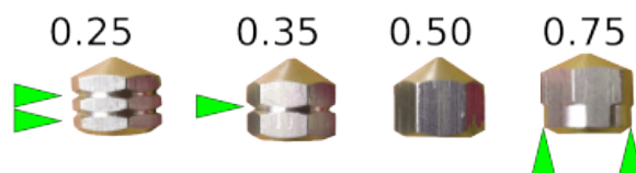
Markings to distinguish nozzle sizes.
