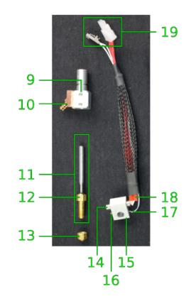
Hot end disassembled
