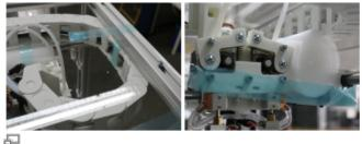
Transport restraint of the main e-chain: blue tape is strapped around the chain an fastened to the top cover.
