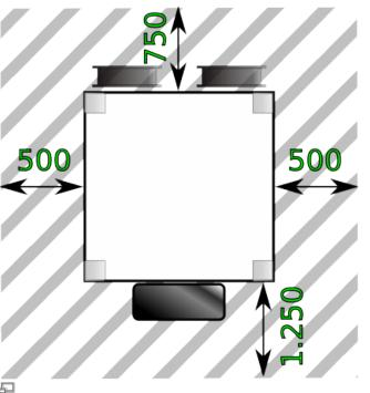
must be left at the back of the RepRap Industrial Necessary free space around the RepRap
