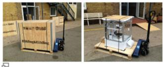
The wooden box and the lid are fastened to the pallet with tensioning straps.
