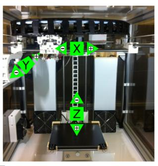
Denotation and direction determination of the axes.
