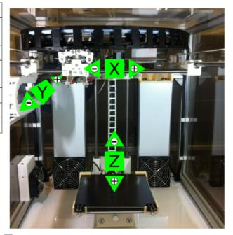
Denotation and direction determination of the axes.
