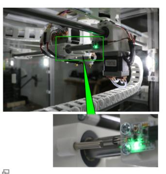
Hall effect sensor and magnet of the X-axis.
