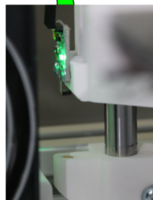
Hall effect sensor and magnet of the Z-axis.
