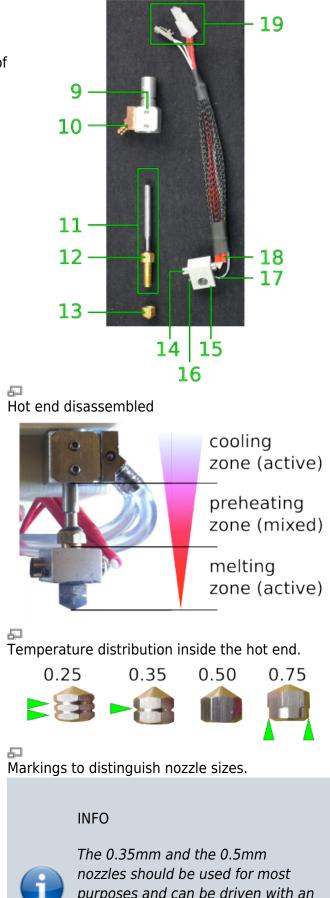
The nozzle is exchangeable to provide different bore diameters for different materials, layer thicknesses or print speed. Ex factory, the 0.35mm tip is preinstalled. Additionally, three nozzles with diameters of 0.25mm, 0.5mm and 0.75mm are included. The tips are distinguishable by the engraved markings.
