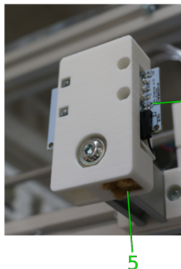
Filament inlet with limit switch and dust wiping
