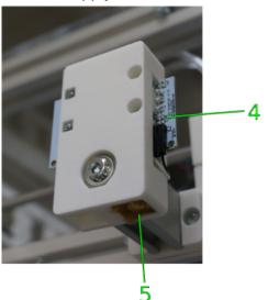
Filament inlet with limit switch and dust wiping
