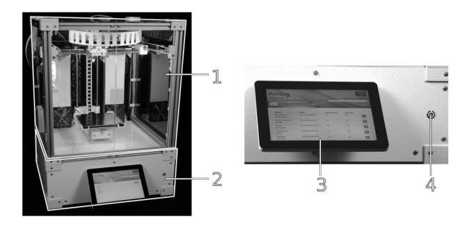
The two main functional sections of the RepRap HMI touchscreen for direct operation and wake Industrial 3D Printer: the build chamber with the button at the front panel. functional components and the electronic chamber containing the regulation electronics.
