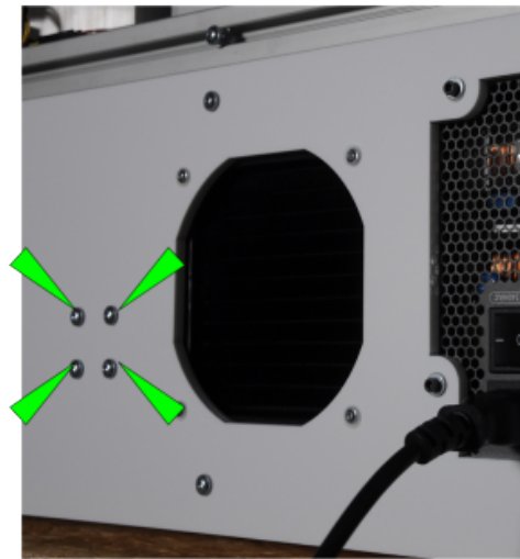
Holding screws of cooling water pump.
