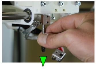
Pull the barrel out of its seat.
