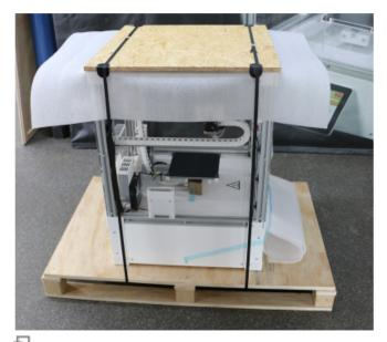
The 3D printer must be tightly secured on the transport pallet.
