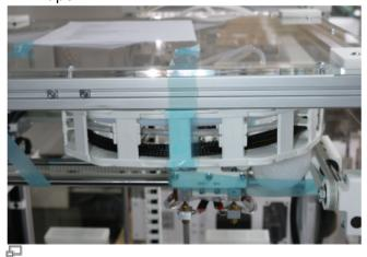
Entwine the e-chain with tape and fasten it to the printer's top cover.
