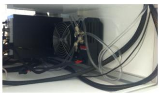
Cooling water pump mounted in the electronic chamber.
