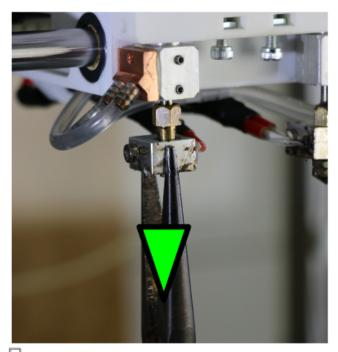
Pulling the heating block off the barrel.
