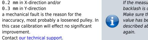
If the measured value is >1mm, backlash is over-compensated. Make sure that the compensation value has been set to 0 as described above and measure
