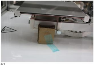
Place the cardboard support underneath the print table and fix it with tape.
