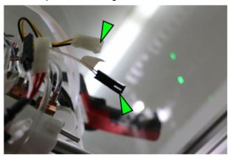
Both connectors must be carefully disconnected.
