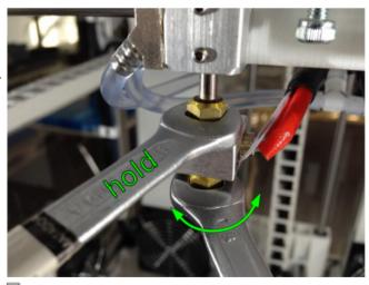
Unscrewing and fastening the nozzle tip requires attention not to overwinde and sheer off the thread.
