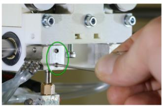
Loosening the hot-end mount set screws is mandatory to avoid breaking the glued connection of barrel and melter.
