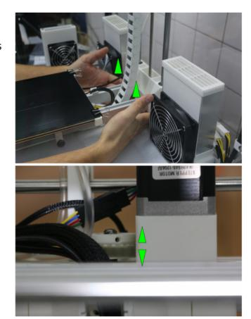
Try to lift the Z-elevator and watch the pulley. If the pulley moves up and down, the clamp collar must be repositioned.
