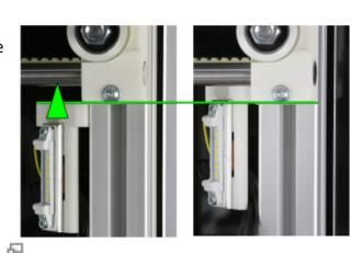
Do not try to hide the LED's supply lines in the groove of the frame. This may lead to damage since the hammerhead nut of the mounting arm must be fastened in the frame groove.
