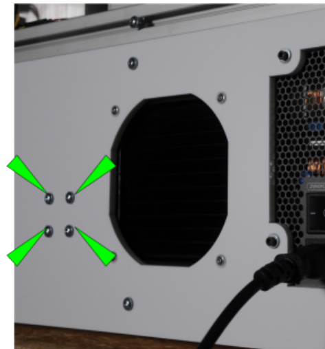
Holding screws of cooling water pump.
