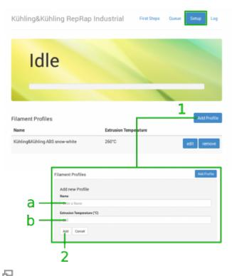
Filament profile setup via the web interface.
