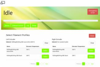
The currently active material profile is also displayed at the start screen of the priming wizard after selecting the extruder that is to be primed.
