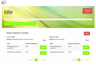
The currently active material profile is also displayed at the start screen of the priming wizard after selecting the extruder that is to be primed.
