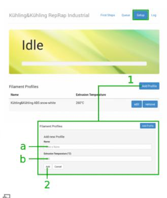
Filament profile setup via the web interface.
