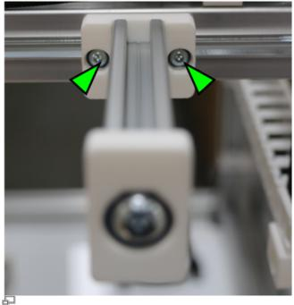
Loosen the fixing screws of the spool carriers.
