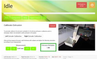
The extrusion multiplier is calculated automatically from the measurement and must be saved in the filament profile of the slicing software.
