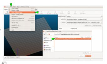
After importing the profile bundles Slic3r is equipped with all necessary presets and ready for operation with the RepRap Industrial 3D printer.
