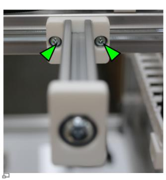
Loosening the fixing screws of spool carriers.
