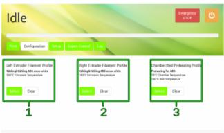
GUI Configuration screen with temperature profile selection.
