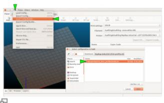
After importing the profile bundles Slic3r is equipped with all necessary presets and ready for operation with the RepRap Industrial 3D printer.
