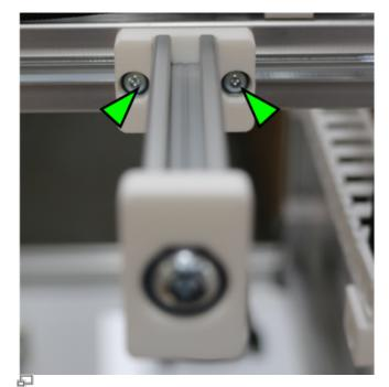
Loosening the fixing screws of spool carriers.
