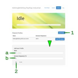
Filament profile setup via the web interface.
