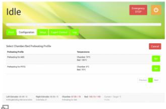
The list of filament temperature profiles of the configuration menu. More profiles can be added via the web-interface.
