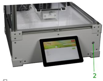
Waking the 3D printer from standby.
