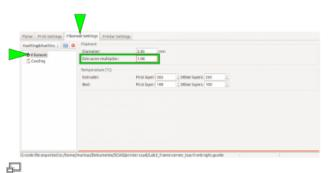
Setting the extrusion multiplier in Slic3r.
