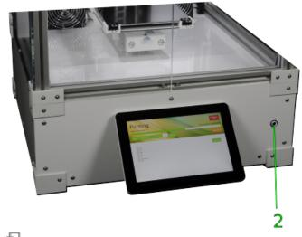
Waking the 3D printer from standby.
