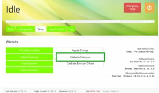
Choose the [Calibrate Extrusion] wizard from the *Setup* menu (either software version).
