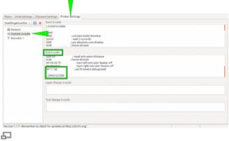
Switching off the build chamber heating
