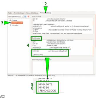
Switching off the build chamber heating elements by modifying the Slic3r custom End Gcode.
