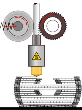
The layer-by-layer build-up of random geometries becomes possible with FFF additive manufacturing machines.
