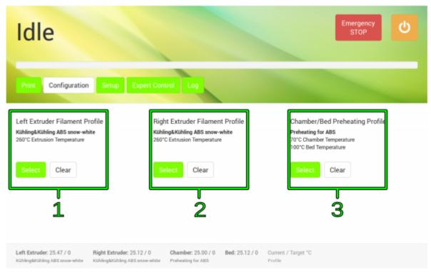
GUI Configuration screen with temperature profile selection.
