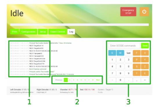
E The log screen provides additional information about sent and received G-code commands and the possibility of directly influencing the 3D Printer via G-code command input.
