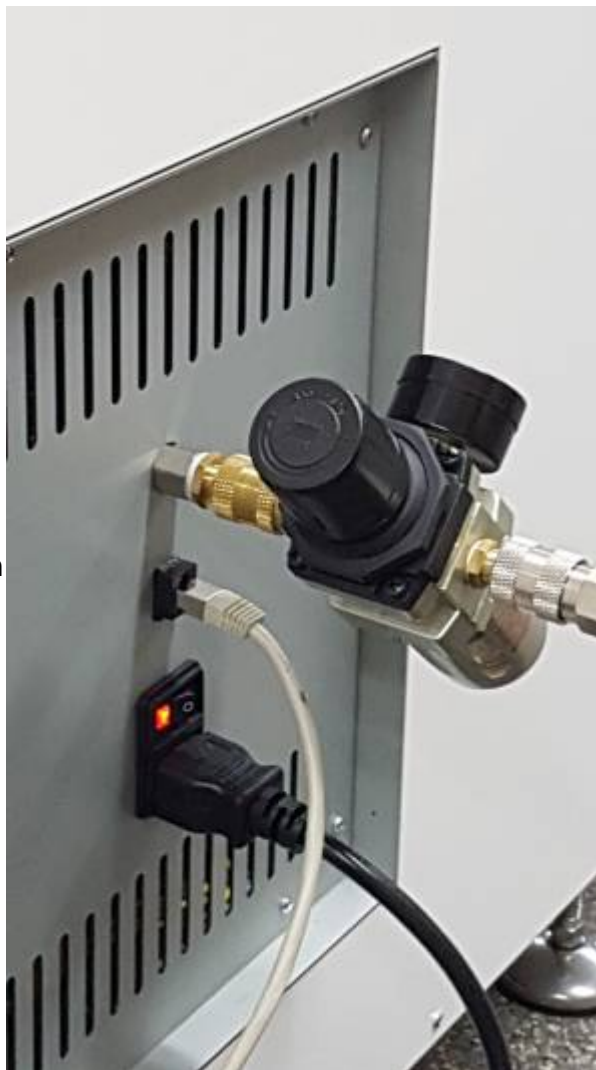
Connections on the rear side of the machine: 230 V power plug, RJ45 Ethernet socket and DN 7.2 pressure reducer.
